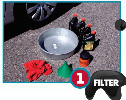
After changing your motor oil, DRAIN oil filter into a drain pan or container for at least 24 hours.
